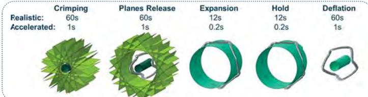
Fig. 2 – Visualization of the five simulation's steps with definition of each step time for both the realistic and accelerated case.
