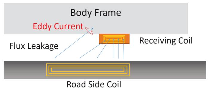
**Flux leakage occurs eddy current loss**
