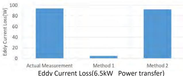
In-Motion WPT system is too big to make mesh model for calculating eddy current accurately enough.
