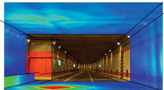
Superposition of the AST maps ("digital Condó road tunnel") and real Condó road tunnel
